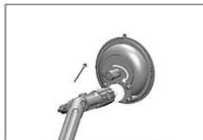
Press the SUCTION BASE on the windshield and tighten the TURNTABLE.
