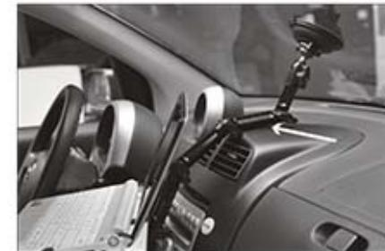
Keep the ARM close to the central console will reduce the vibration.
