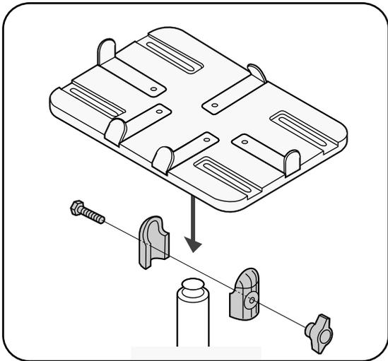
\* Screw the holding plates tightly to the ball.
